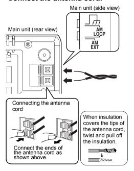
3 Turn the AM loop antenna to find the best position for radio reception.
